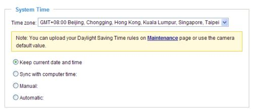
Keep current date and time: Select this option to preserve the current date and time of the Video server. The video server's internal real-time clock maintains the date and time even when the power of the system is turned off.
